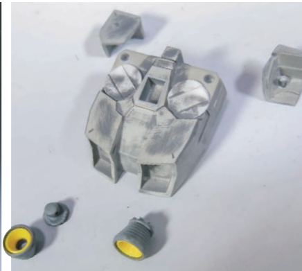
▶ The hip's base was box-assembled. Except for the ball joint from the kit, I made the armor out of epoxy putty. I drilled a crotch connection hole for an action base. In addition, I created a lid and an adapter part for an action base.
