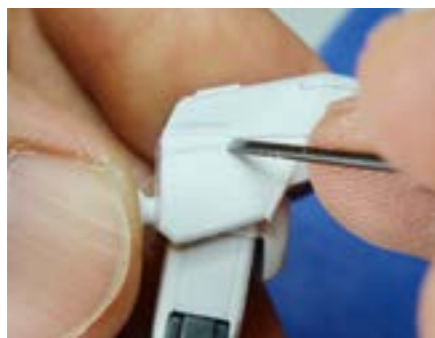
▲ Next, I will engrave the lines of the part to be made into a recess. For short sections, I will use a chisel to create a V-shaped groove.
