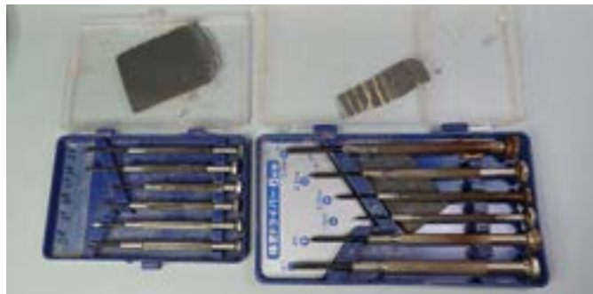
▲ This is also an indispensable tool for model making. Homemade engraving blades made by sharpening the tip of fine dollar-store screwdrivers with a whetstone! I find them invaluable for tasks such as carving recesses, scraping lines, polishing with the edge, and more. The extremely thin one is a special item made by further modifying one with a grinder!
