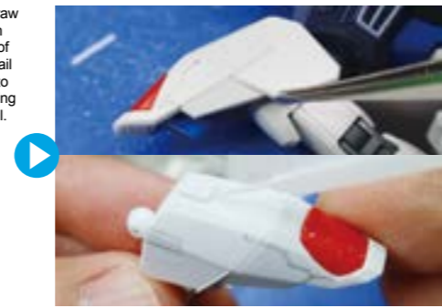
▲ I attach a plastic plate to the part I want to make into a convex detail.
