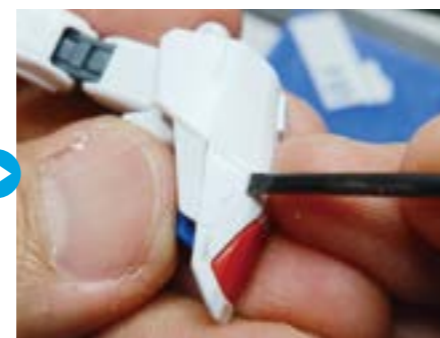
▲ I will do the same with the other grooves, engraving along the pencil marks.
