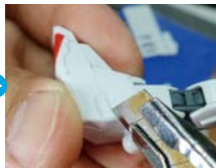
▲ For lines that are longer than the length of the chisel, I'm going to use a cutter to make them V-shaped.
