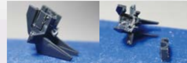
▲ To adjust the proportions, I shortened the neck joint. To lower the poly cap mount on the neck, I cut out a piece.
