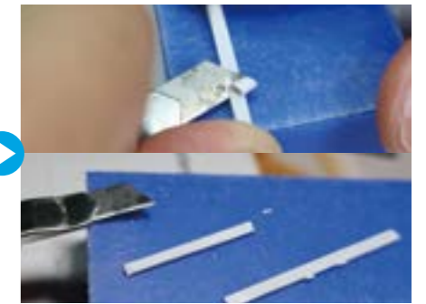
▲ Making a runner into a flat shape. I shave it to flatten one side with a cutter, then shave the opposite side using the first side as a reference and turn it into a flat shape.
