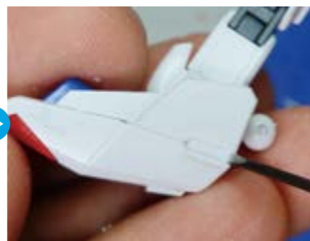
▲ I am going to use the grooves I added as a guide to engrave the inside of the surface with a chisel one step lower.
