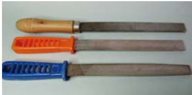
▲ While I've been hesitant to overuse my higher-end metal files, the ones I've had the most success with are, surprisingly, from a dollar store. They've proven invaluable for flattening the runners. In fact, aside from recently replacing the second orange one, I've been using the same files continuously since my debut. Their longevity is impressive, to say the least. The blue patterned file has a semi-rounded shape.
