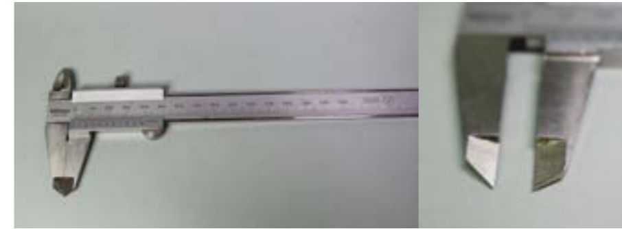
▲ These calipers are made of metal. I sharpened the tips with a grinder to make scraping and shaving details easier.
