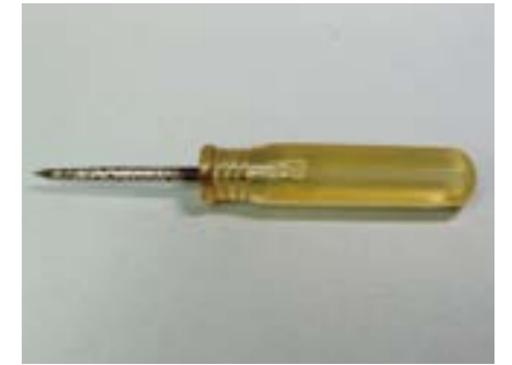
▲ Needle-nose screwdrivers are a common item in driver sets. I make good use of them for tasks such as re-carving panel lines and dotting circular detail points. I sharpened the tip to a fine point with a metal file.
