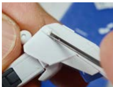
▲ I am going to use the grooves I added as a guide to engrave the inside of the surface with a chisel one step lower.
