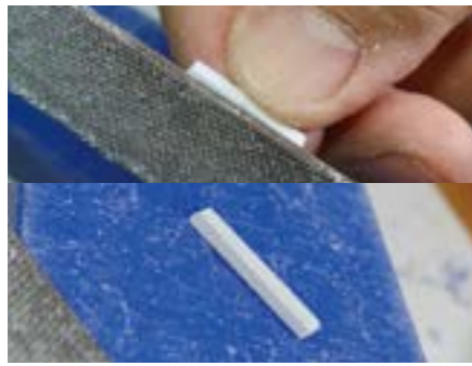
▲ To give the front hip armor the same volume, I will also attach thicker runner plates to adjust it. I chamfered them first before attaching them.
