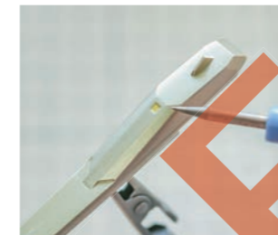
▲ I cut the tape. You can see that it covers all the way to the edges of the concave mold. The method of cutting the tape directly on the part allows you to mask even complex shapes once you get used to it. I'll say it again, I don't recommend this method for beginners. (urahana3)
