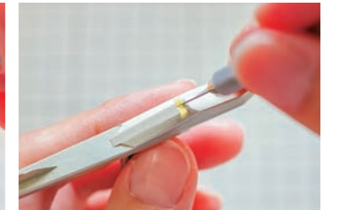
▲ Using the scored lines in the last step as a guide, trim the excess masking with a precision knife. Drawing a shape on the masking tape and cutting it on a cutting mat can result in slight misalignment, so cutting directly on the part ensures a perfect result. However, it takes some practice to master the right amount of pressure, so it is not recommended for beginners. (urahana3)
