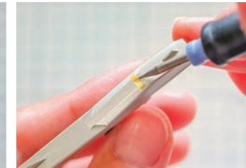
▲ Mask the concave mold. Apply masking tapes of equal width to the top and bottom, making sure to draw visible lines by scoring the left and right sides with a scribe.
