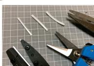
$\blacktriangle$  Compare cut edges. Observe the cut edges of plastic sheets cut with different tools. Thinner cuts typically show more curvature. But the Amazing Cutter stands out! It produces remarkably clean, straight cuts, even on thin sections. In fact, this tool is so enjoyable to use, you may find yourself cutting more than you need to.
