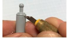
▲ Recarving recessed shapes is also easy with a design knife or art knife. With just one more step, you can even create new panel lines!
