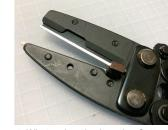
▲ What makes the Amazing Cutter a knife? The "blade" is a replaceable razor blade, the same type used in utility knives. When the blade dulls, you can simply replace it, restoring the sharpness and allowing you to continue slicing through plastic sheets with effortless precision.
