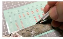
▲ The true purpose of a knife is to cut. When it comes to trimming excess decal material, design knives are the clear winners. Their angled blades provide a clear view of the cutting line, making them the perfect tool for precise detail work.
