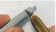
▲ After making a double cut on the gates, you can use an art knife to remove the nubs. This is especially helpful if you find nippers a bit tricky to control. Just be careful and watch where the blade is going to avoid accidents.
