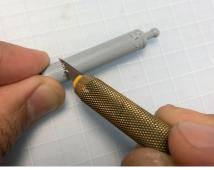
▲ When it comes to tackling those pesky nub marks, ▲ Rather than using only the tip, use the "belly" of the art knife – the curved area just behind the tip – to plane and smooth the parting line. Apply gentle, even pressure as you glide the knife in a forward motion
